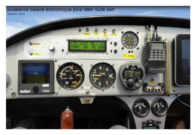
Economic speed, for the sake of a relaxing flight, 175k/h (94.5 knots) from 5 to 5.5 l/h (from 1.32 to 1.45 USG).
