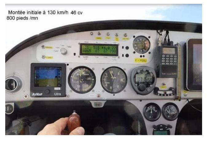
Initial climb: 800 ft/mn at 70 knots, the engine delivers 46 hp (4065 rpm).
