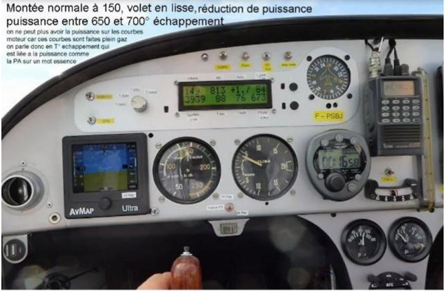
Power reduced (3939 rpm), zero flaps, and normal climb 500 ft/mn at 81 kt.
