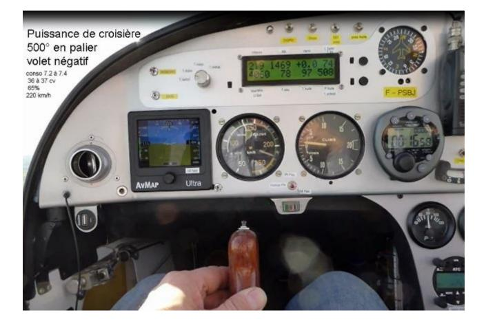
Level flight, the engine delivers 36 or 37 hp, 65% power 7.5 l/h (1.98 USG) at 220 km/h (119 knots).
