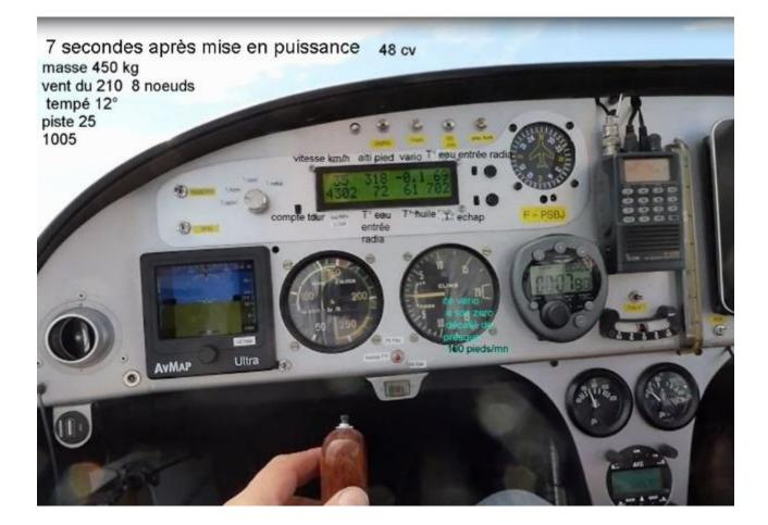
The picture above shows that after about 7 seconds (round clock under the aircraft registration) after applying full throttle the engine delivers 48hp at 4302 rpm.
