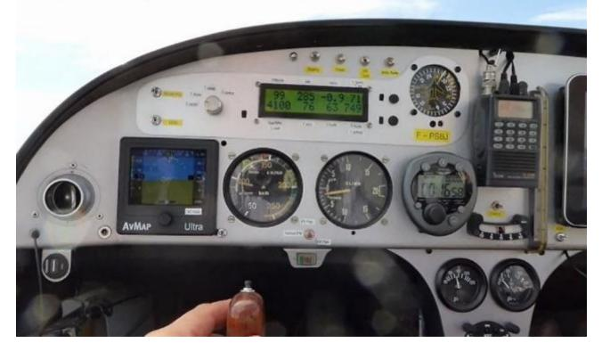
Above: The rotation speed is reached after 16"58 and a 688ft takeoff roll. Note: Variometer should read 0 but it shows an offset of 100 feet and reads -0.1.
