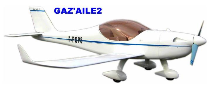
The picture below shows the first aircraft built in collaboration with my friend Lucas back in 1998. We achieved our goal in putting in flight a successful operational aircraft using a turbo diesel engine (Opel Corsa) that delivered 68 hp.
