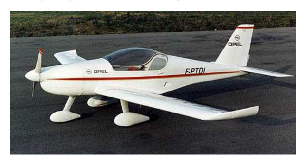
I then came out with the very first ultra-light equipped with a diesel engine (a Citroen AX engine mounted on drastically modified Rands COYOTE).
