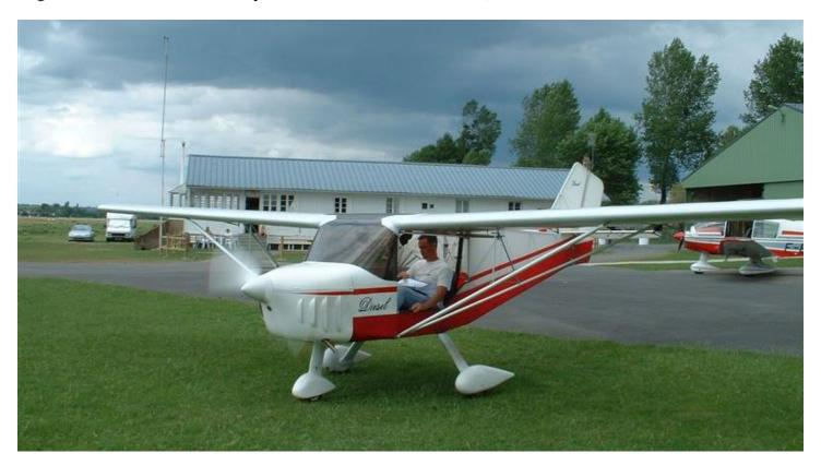
I then improved my first diesel aircraft and I baptized it GAZ'AILE 1; the engine mounted on this enhanced version was an Isuzu turbo diesel developing 85 hp.
