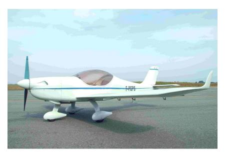
Below is the first was the first in recent years (1998) myself and in collaboration with my friend Lucas, we achieved a successful and operational demonstrator diesel aircraft with a diesel engine (engine Opel Corsa).
